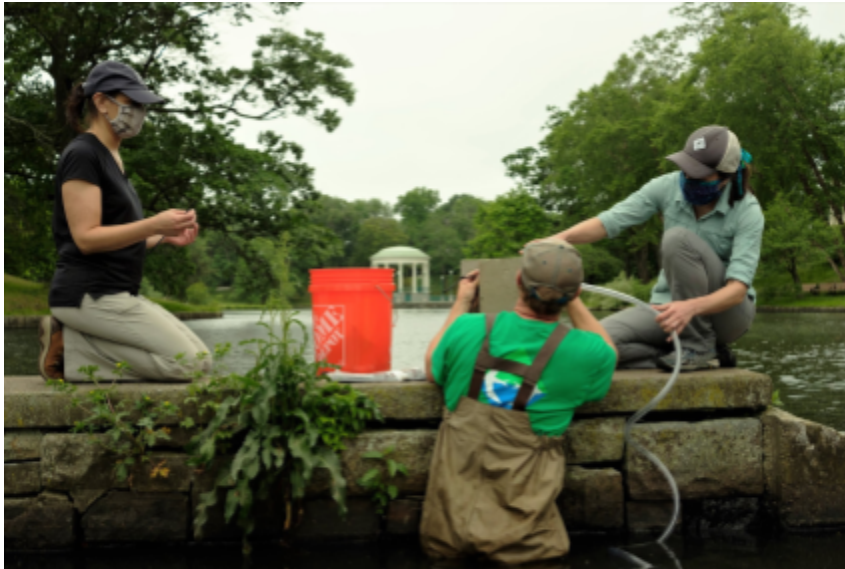
Ryan Kopp (Audubon Society of RI), Kelly Addy (URI) and Elizabeth Buschert (UNH) install intake tubing for a continuous nutrient monitoring system.
